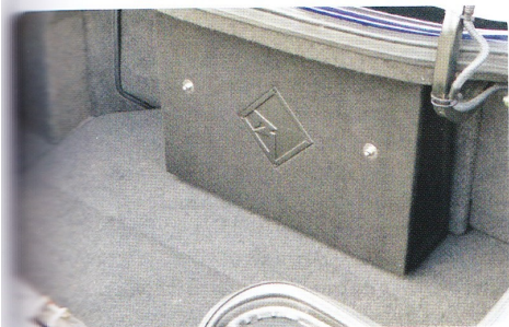
The new subwoofer ducted over the fuel tank and into the car occupies surprisingly little boot space
