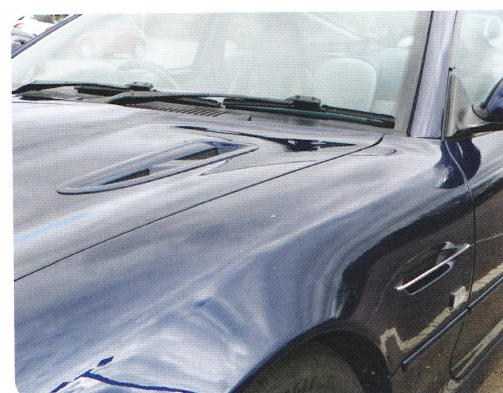
The modified Jaguar vents and new low profile wipers and 'normal' washer jets
