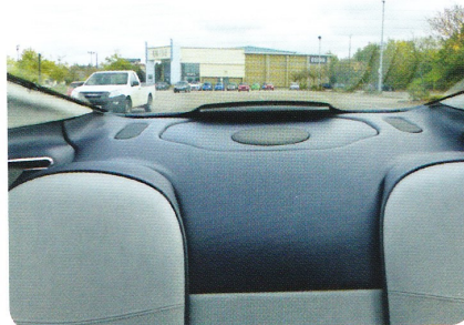
The grille for the ducted subwoofer was chosen, finished and fitted to look as original as possible
