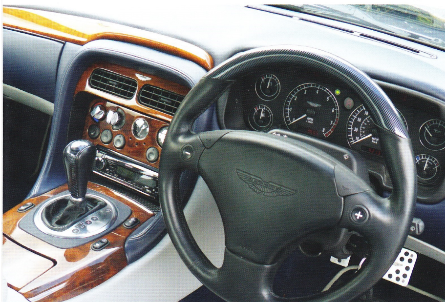
The black plastic gear surround has been changed to something more 'durk tecknik'. Note the new indicator tell-tale light glowing in the instrument cluster
